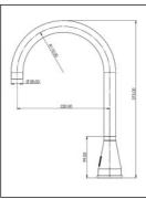
Non-contact self-closing DN 15 Washtable-tap, stainless steel satin; with rotating and lockable curved spout, aerator\*, optosensor. For premixed water (UT mixer).
